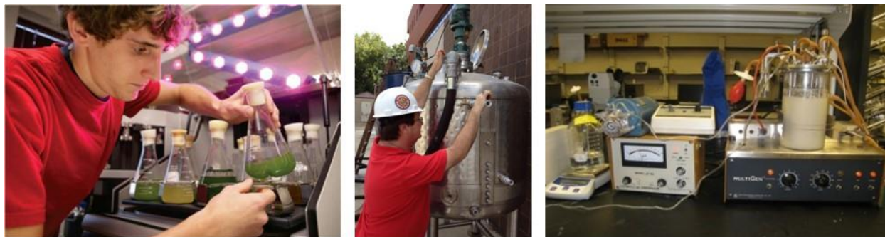
(L to R) Culturing Microalgae, Pilot Scale Anaerobic Digester, & Production of Lipids from Yeast
