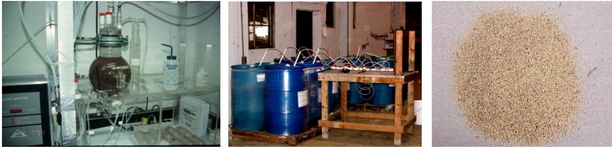
(L to R): Bioslurry treatment of contaminated soil, insitu chemical oxidation using Fenton's Reagent, and development of a kenaf-based adsorbent
