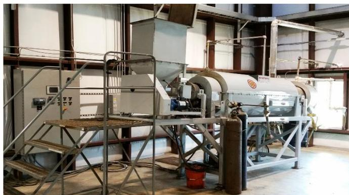
Second project involves evaluation of process operational parameters on production of densified bio-coal from bagasse, using reactors at all scales; bench, pilot (10 kg/hr) and demonstration (2 tons/hr) in collaboration with American Biocarbon. In addition, this project aims at evaluating critical design data (such as heats of torrefaction).
